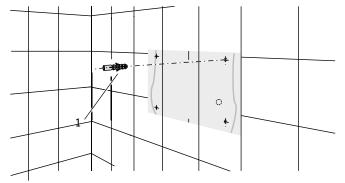
Secure the unit into the pre-drilled holes.
