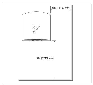
Mount the hand dryer at least 48  $^{\prime\prime}$  (1219 mm) above the floor.
