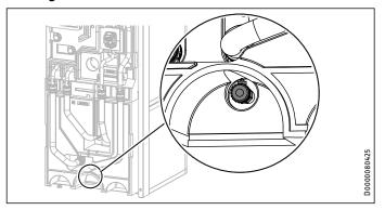
▶ Drain the buffer tank via the drain valve.
