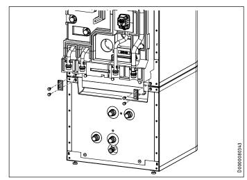
► Release the 4 screws on the tabs at the front of the appliance.
