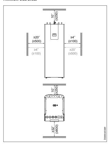
The minimum side clearances can be swapped between left and right.
