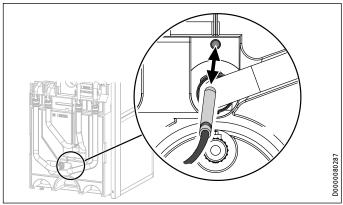
▶ Pull the "heating sensor" out of the buffer tank.
