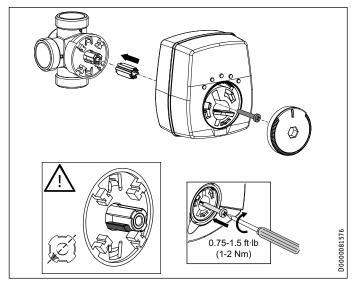
► Check the position of the 3-way mixer shaft.
