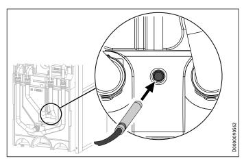
Insert the temperature sensor into the sensor well "Sensor heat pump cooling, optional".
